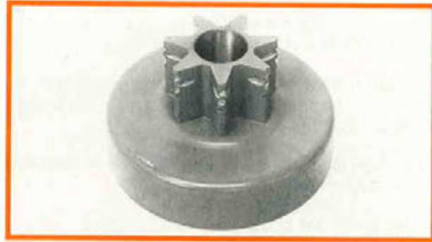
Worn chain sprocket
