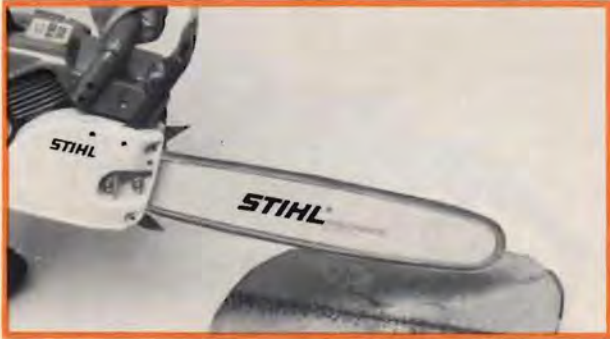
Checking chain lubrication
